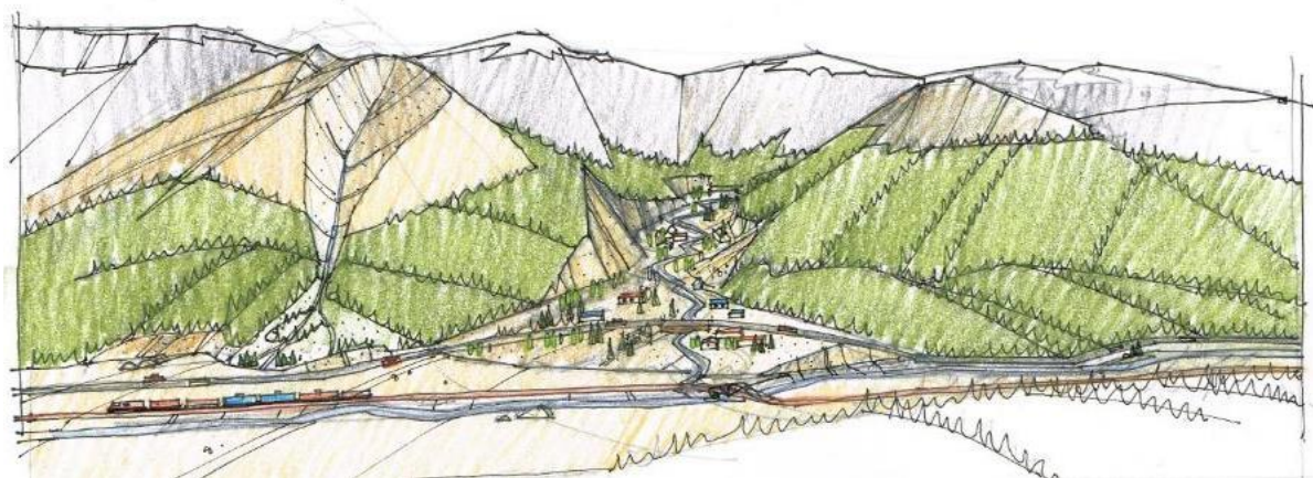
Figure C-3. Typical steep and low-gradient fans feeding into a broader floodplain. On the left a small watershed prone to debris flows has created a steep fan that may also be subject to rock fall processes. On the right a larger watershed prone to debris floods has created a lower gradient fan. Development and infrastructure are shown to illustrate their interaction with steep creek hazard events. Artwork: Derrill Shuttleworth.
